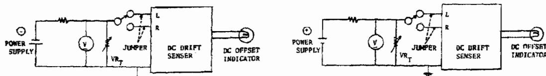
Check (+) and (-) voltage respectively for both channels. It is all right when it is within  $\pm 450\text{mV}$ .
